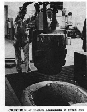
of the furnace by using overhead crane. Performing the operation are Donald Quayle, left, and Wilfred Sanchez. Sandia furnaces do not have large exhaust hoods over the furnaces that are common to most foundries, instead a steady stream of air is blown across from duct at left, sucked out by a duct on right.
